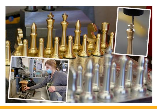
Students in MCH351 CAD CAM Applications class have been very busy designing and machining a very remarkable chess set. The students designed all the parts using Fusion 360 then machined all of the parts using a CNC lathe and milling machine. The pieces were made out of brass and aluminum.
